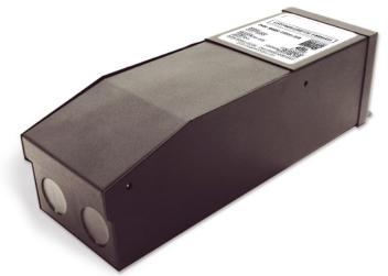
KLUS - MD-100-12 is the most compact LED driver on the market with a magnetic transformer core. It is equipped with two auto-reset breakers, one on the input and one on the output, which protect both the load and driver. The driver is encased in a coated metal. box that includes 2 knock-outs, one on each side, to enable easy installation that complies with electrical code requirements.
